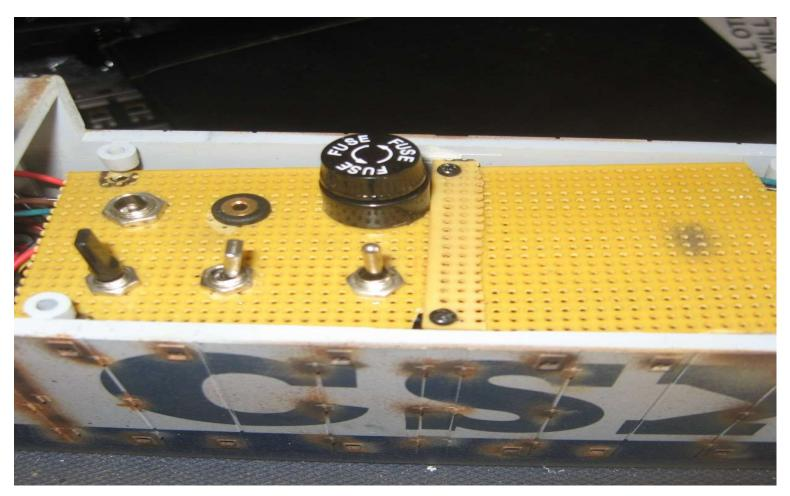
Here is the control switches. Upper left charging jack, Phoenix computer interace, fuse. Lower left switch is a center off. Switch to left your on battery to the right your on track power. Center switch is for turning off the sound board durning programming of CV's . Switch on right controls volume of sound system. Bob Conant has the following for sale. He can b reached at
