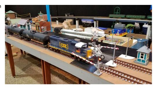
seven Arduino processor modules, with appropriate interface LED driver modules, all triggered by laser track sensors from Model Train Technology Co. who also manufactured the signals and crossing gates.
